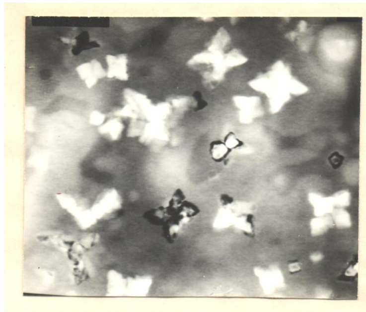
Figure 13(a) TEM micrograph showing Dendritic \alpha -Fe crystals in an amorphous matrix of amorphous \text{Fe}_{67}\text{Co}_{18}\text{B}_{14}\text{Si}_1 alloy (S2) heated to 670 K.
