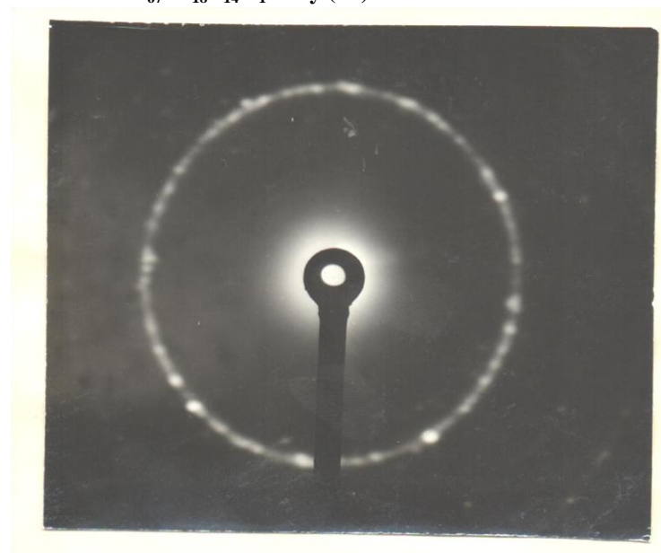
Figure 13(b) The SAD pattern of Fig. 13(a).
